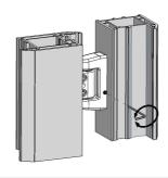
Adjust sash as required using a 5mm allen key.
