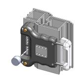
2. Fit 'mounting block' to frame and secure with two Ø4.8x45mm screws provided.
