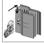
Rotate the 'hinge flag' and engage pegs in pre drilled holes. Secure with two Ø4.8x29mm and four Ø4.8x45mm screws provided.
