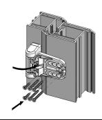
Open the door sash and engage to anti lift off screw using a 2mm allen
