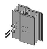
3. Locate 'hinge assembly' on to the 'mounting block' and slide down to retain. (Hinge should slide approximately 14mm to fully engage).
